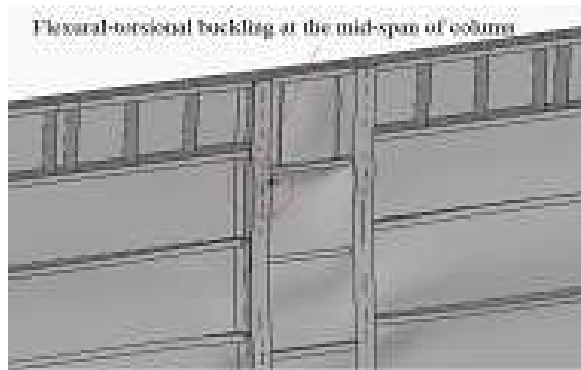
Fig. 4. Buckling mode of the column
